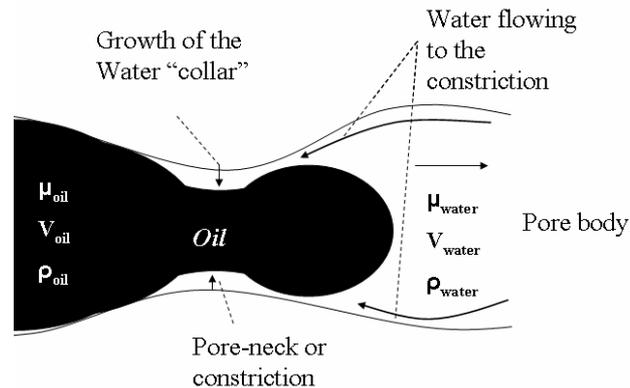
Figure 1. Snap-Off mechanism in a porous media for a system having water as continuous phase.
