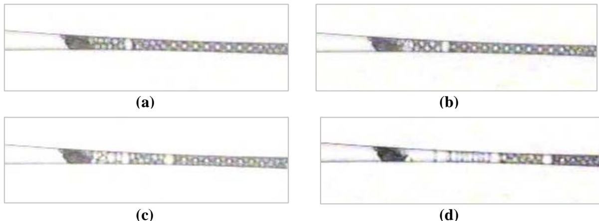
Figure 8. Snap-off during continuous phase running out.
